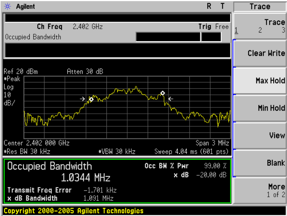
TEST PLOT OF BANDWIDTH FOR LOW CHANNEL
