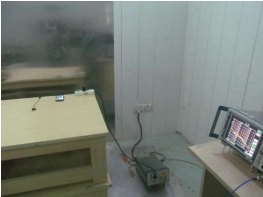
FCC RADIATED EMISSION TEST SETUP
