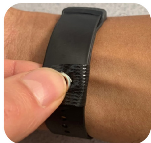
Figure 3.9 Securing the rivet on the WW Tag
