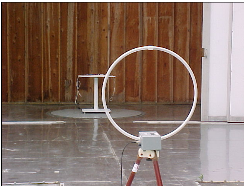
View of the EUT during Radiated Emission Testing on the 10 Meter OATS, measurement of Low Frequency Signals
