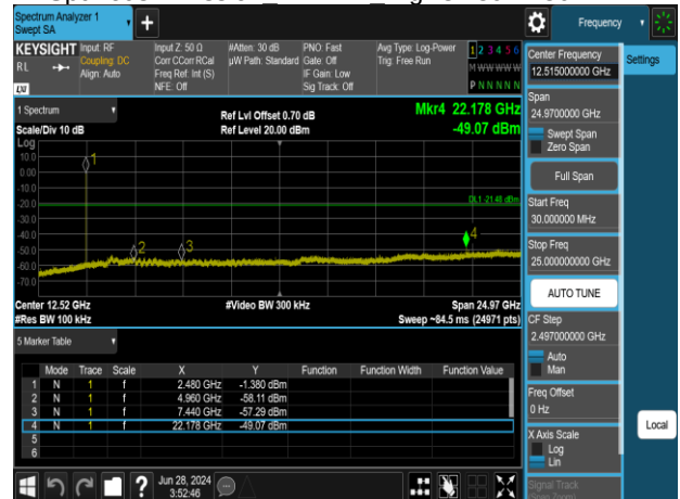
Spurious Emission BLE 2M HighCH39-2480MHz
