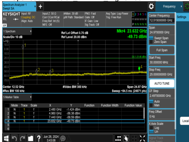
Spurious Emission BLE 1M HighCH39-2480MHz
