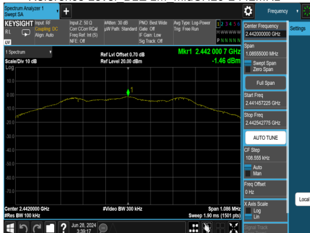
Reference Level BLE 1M HighCH39-2480MHz
