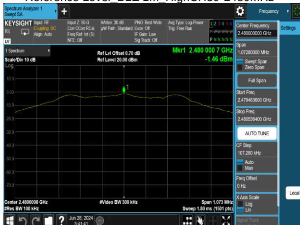
Reference Level BLE 1M HighCH39-2480MHz
