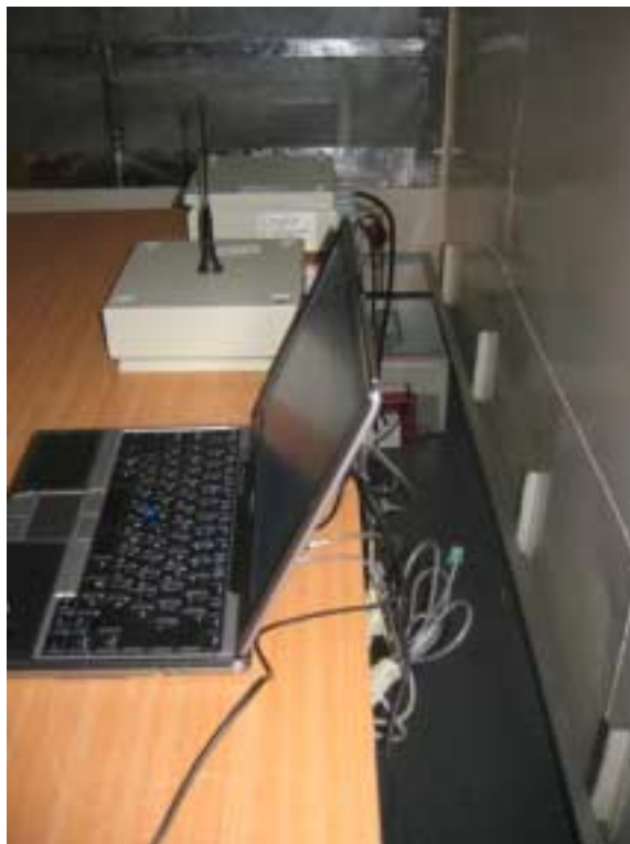
Photograph No.8 Conducted emissions measurement setup
