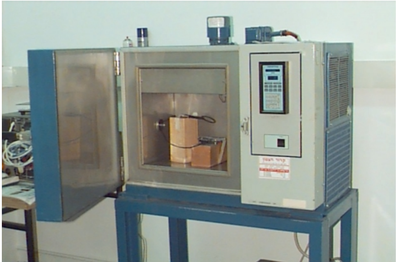
Photograph 6 Frequency tolerance test setup
