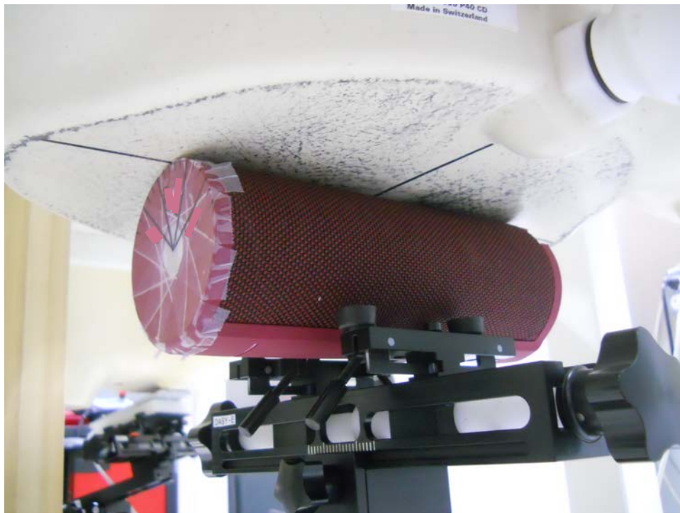
Test Setup Photo 4: Side at 0.0 mm (2.4 GHz WLAN Chain1)
