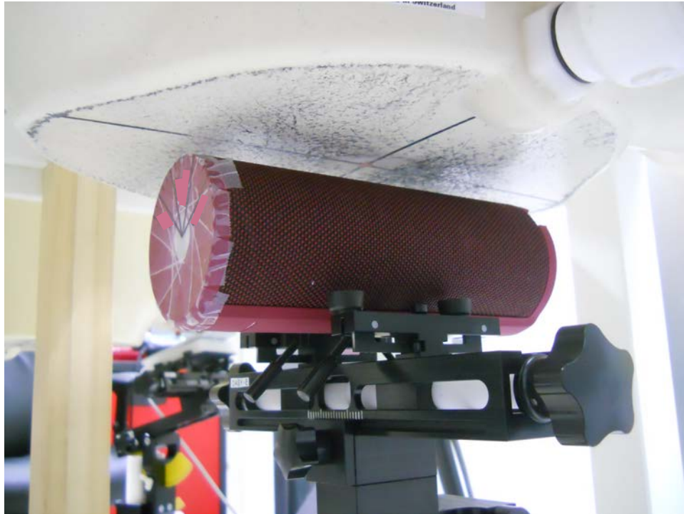
Test Setup Photo 3: Side at 1.0 mm (2.4 GHz WLAN Chain1)
