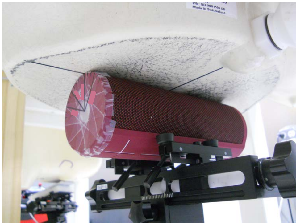
Test Setup Photo 2: Side at 0.0 mm (2.4 GHz WLAN Chain0)
