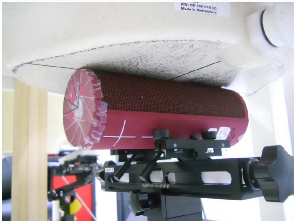
Test Setup Photo 8: Side at 0.0 mm (5 GHz WLAN Chain1)
