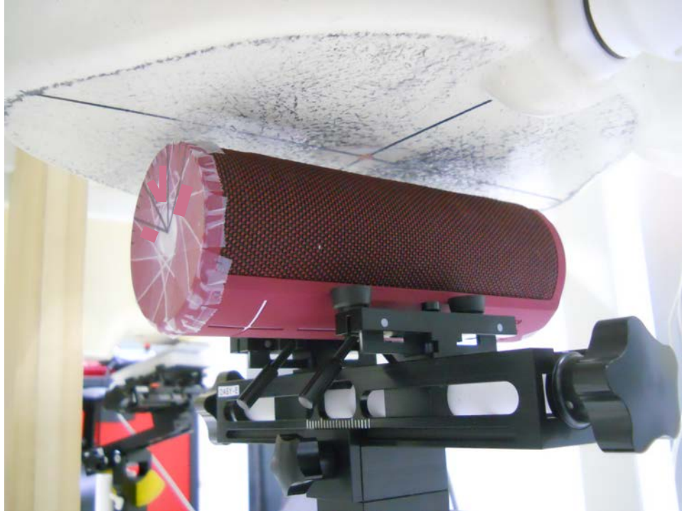
Test Setup Photo 1: Side at 1.0 mm (2.4 GHz WLAN Chain0)
