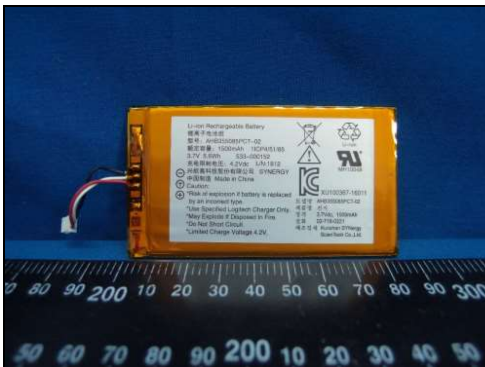
Battery 2 (Model: AHB355085PCT-02 or 533-000152)
