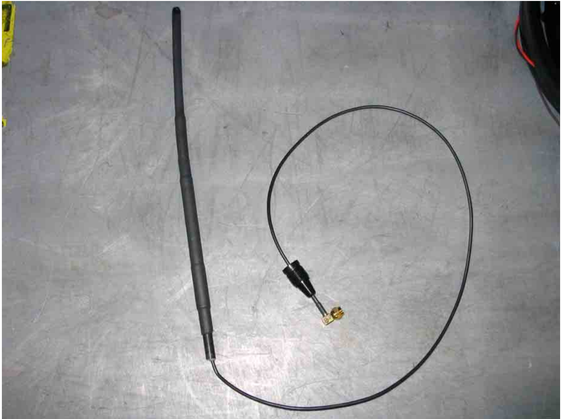
Figure 5: Sleeve Dipole Antenna with Connecting Cable
