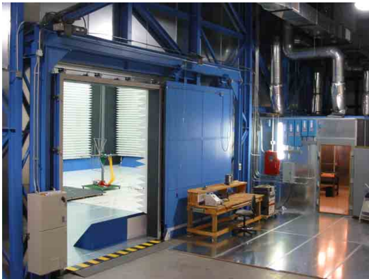
Figure 3-1: 10-Meter EMC Site
