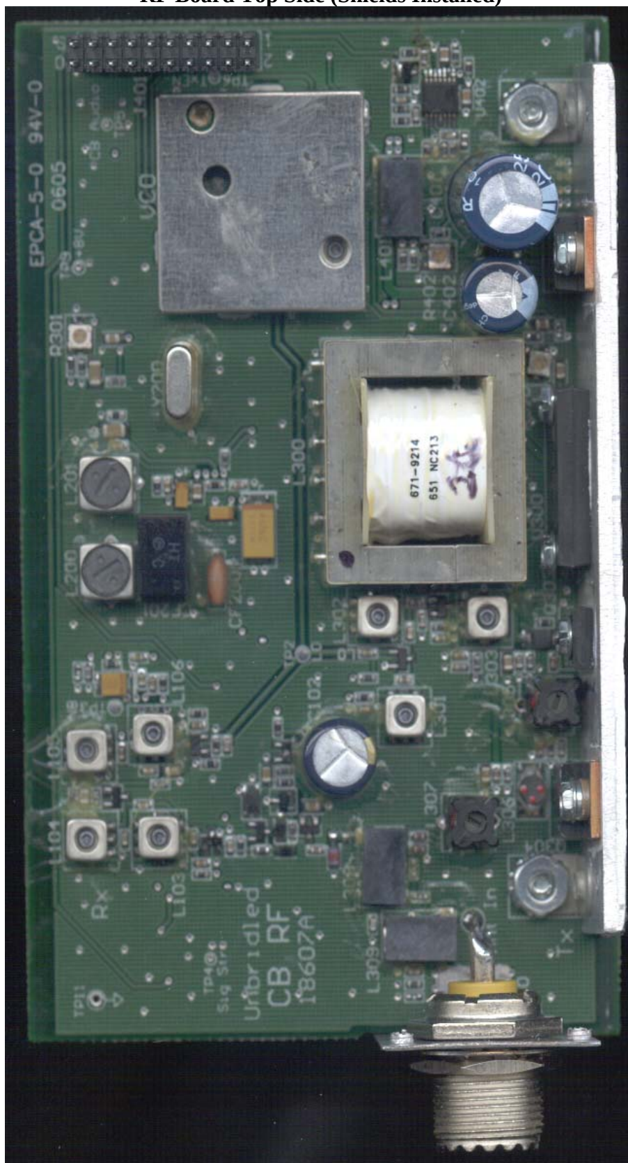
RF Board Top Side (Shields Installed)
