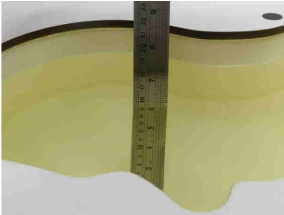
Fig 11.1 Photo of Liquid Height for Head SAR
