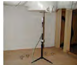
Figure 11.1 Dipole Verification Test Setup Diagram & Photo
