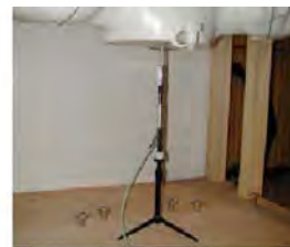
Figure 11.1 Dipole Verification Test Setup Diagram & Photo
