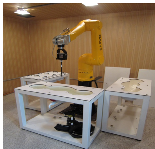
Figure 4.1 DASY5 Test System
