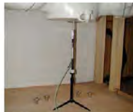
Figure 11.1 Dipole Verification Test Setup Diagram & Photo
