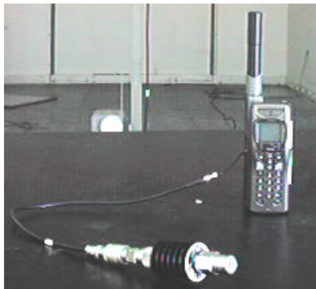
Picture of DUI Configuration in Open Area Test Site (OATS)
