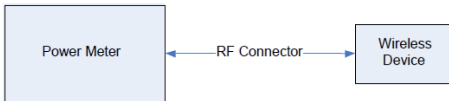
Figure 10.4 Power Measurement Setup
