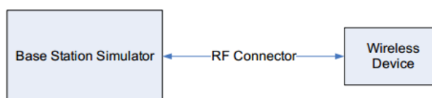
Figure 10.1 Power Measurement Setup
