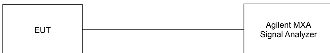
Figure 10.4 Power Measurement Setup for Bandwidths &gt; 50 MHz
