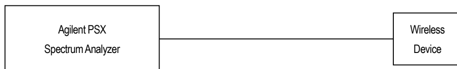
Figure 10.4 Power Measurement Setup for Bandwidths > 50 MHz
