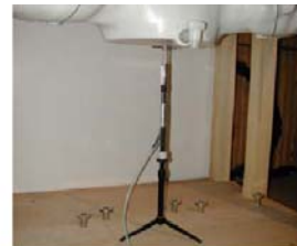
Figure 11.1 Dipole Verification Test Setup Diagram & Photo
