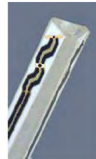
Figure 3.3 Probe Thick-Film Technique
