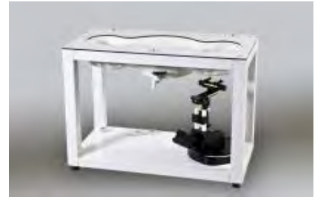
Figure 3.6 SAM Twin Phantom
