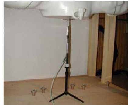
Figure 11.1 Dipole Verification Test Setup Diagram & Photo
