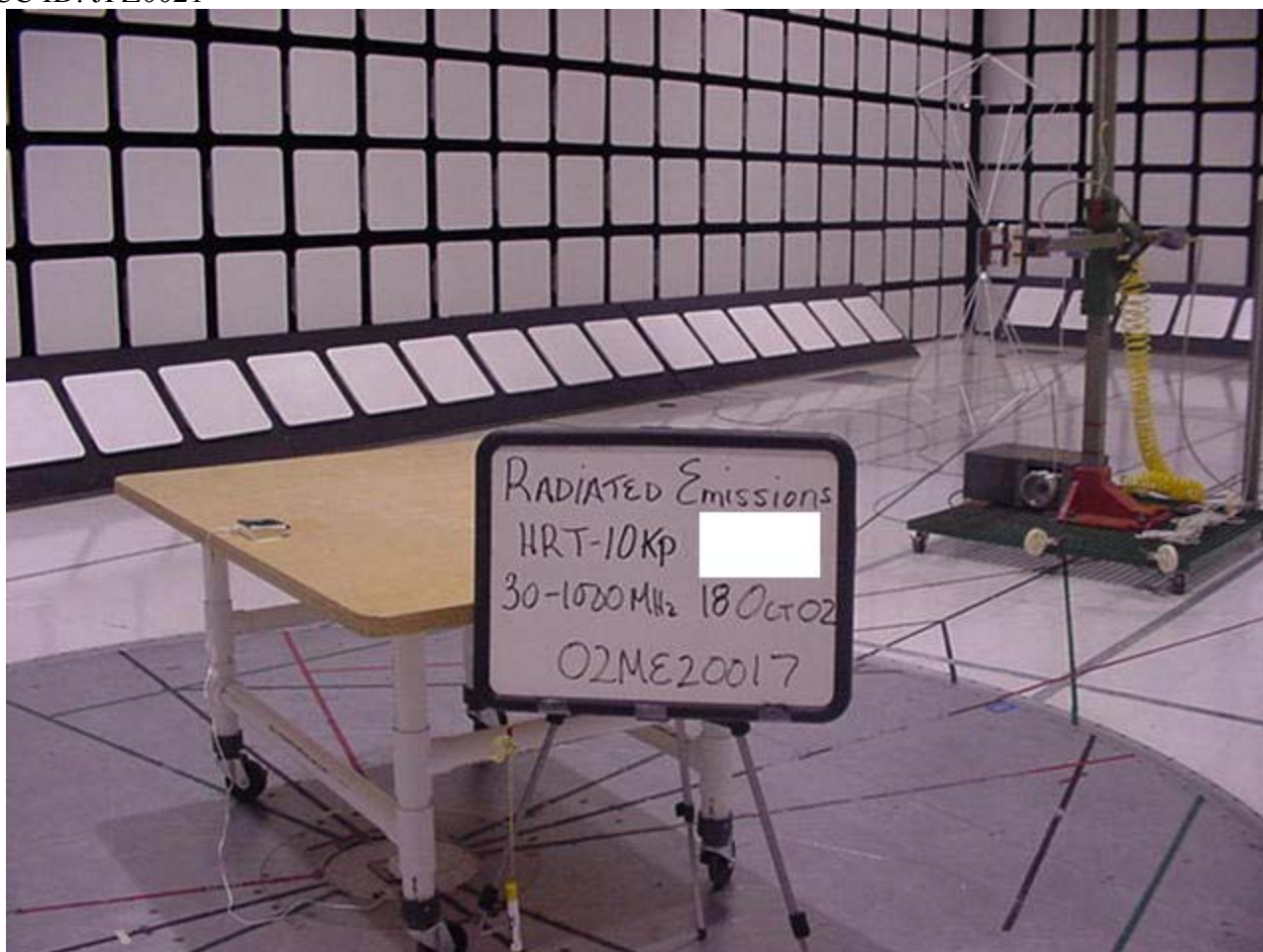
Radiated Emission Test Set-Up 30-1000MHz Front View
