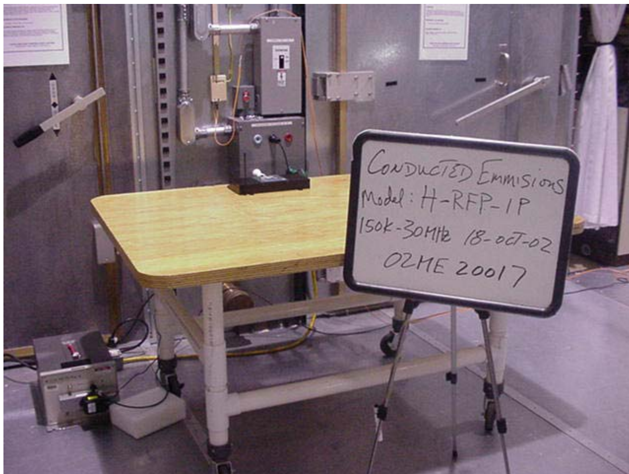
Conducted Emission Test Set-Up 150k-30MHz
