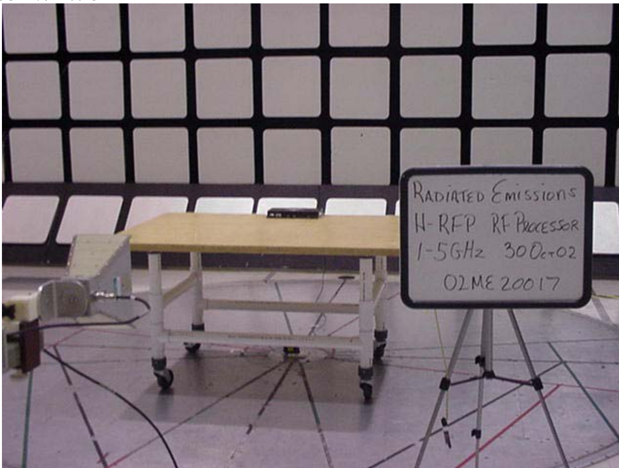
Radiated Emissions Test Set-Up 1-5GHz Front View (Model number in title block H-RFP = H-RFP-1P)
