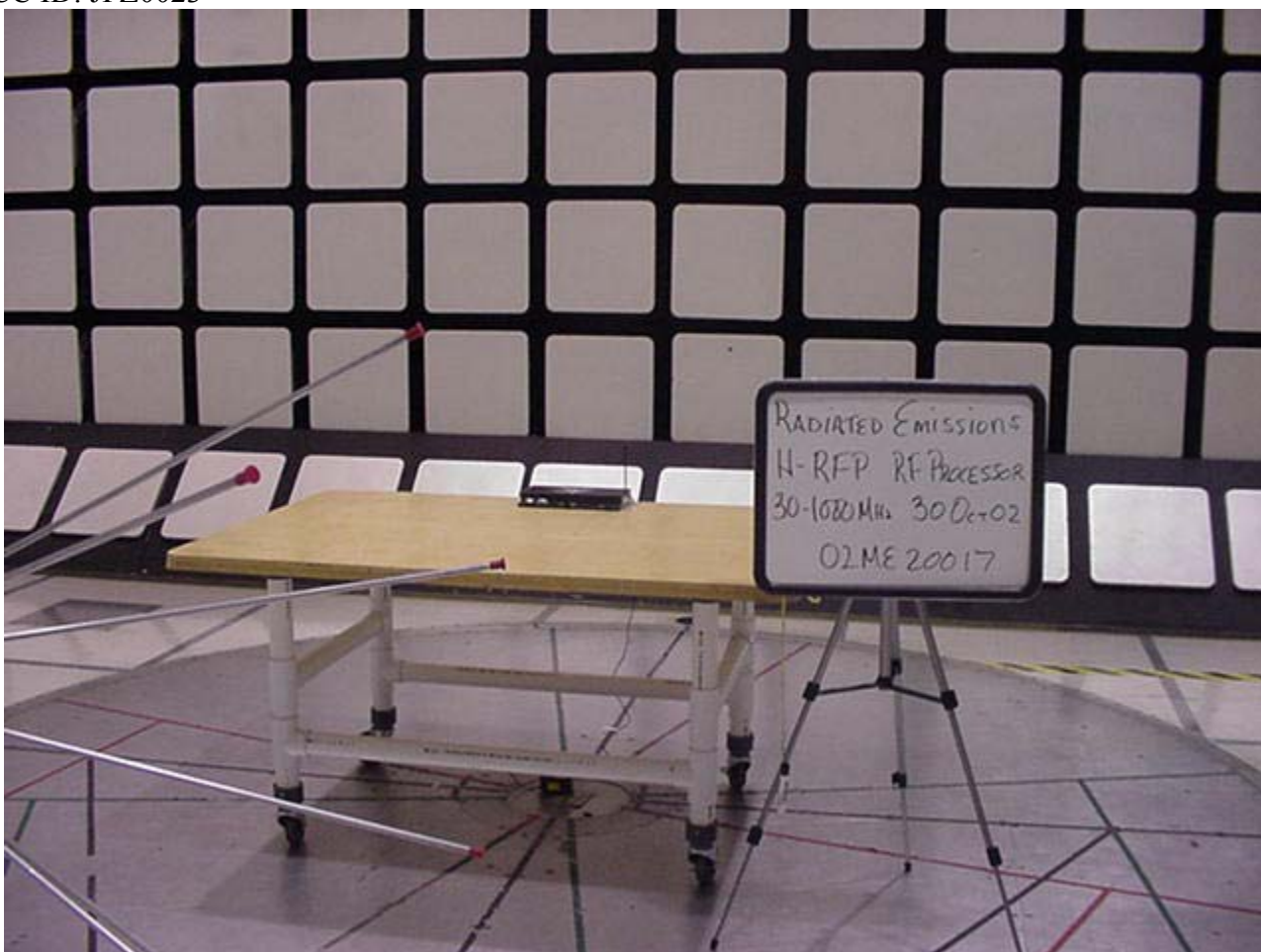
Radiated Emissions Test Set-Up 30-1000MHz Front View (Model number in title block H-RFP = H-RFP-1P)
