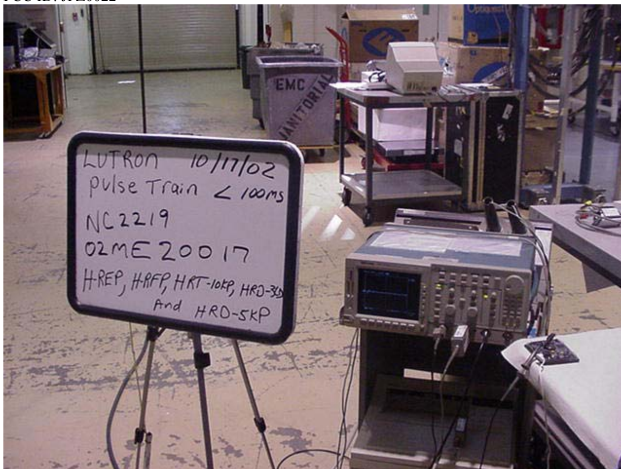
Pulse Train Test Set-Up
