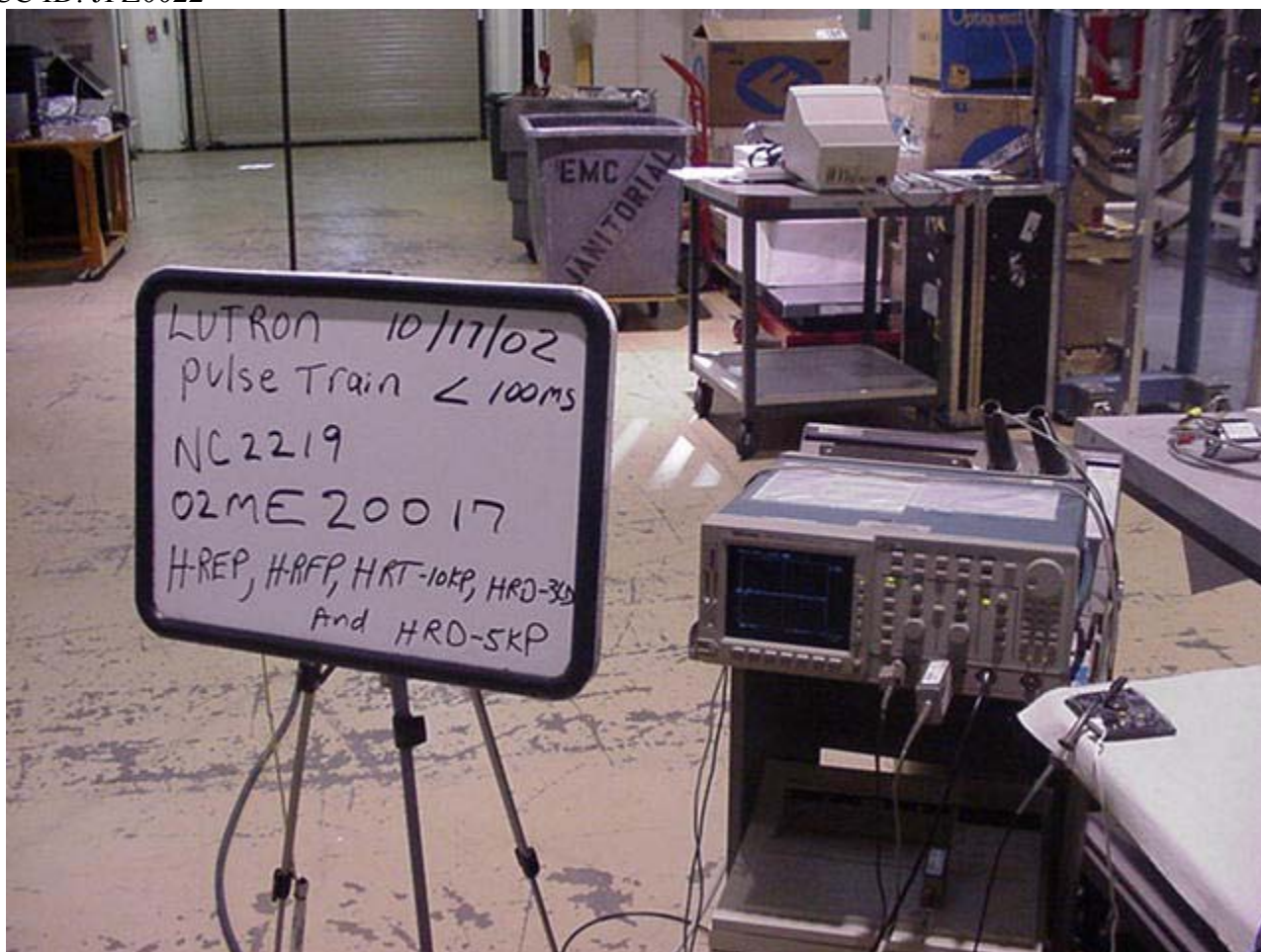
Pulse Train Test Set-Up
