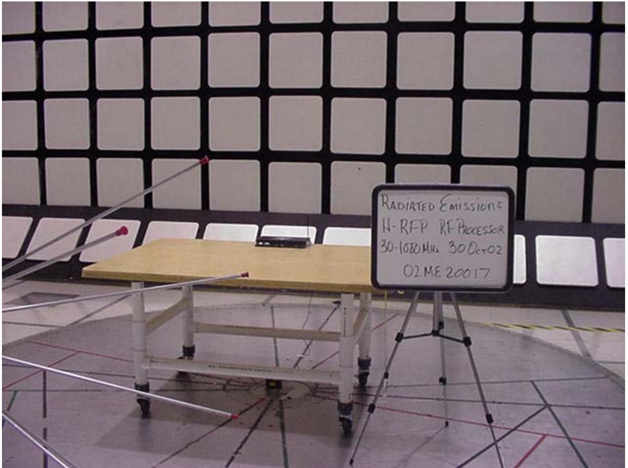
Radiated Emissions Test Set-Up 30-1000MHz Front View
