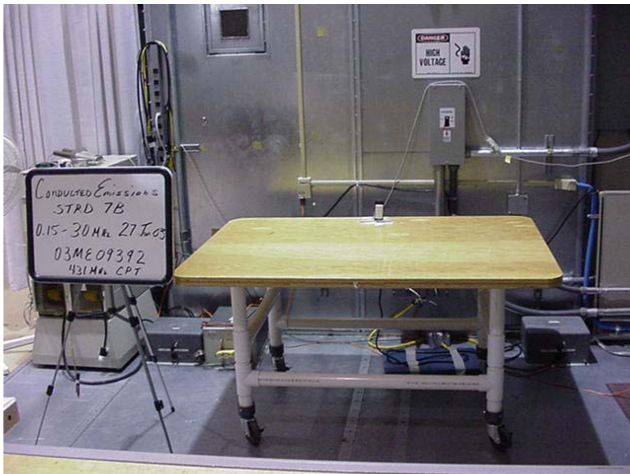
Conducted Emissions Test Set-Up 150k-30MHz
