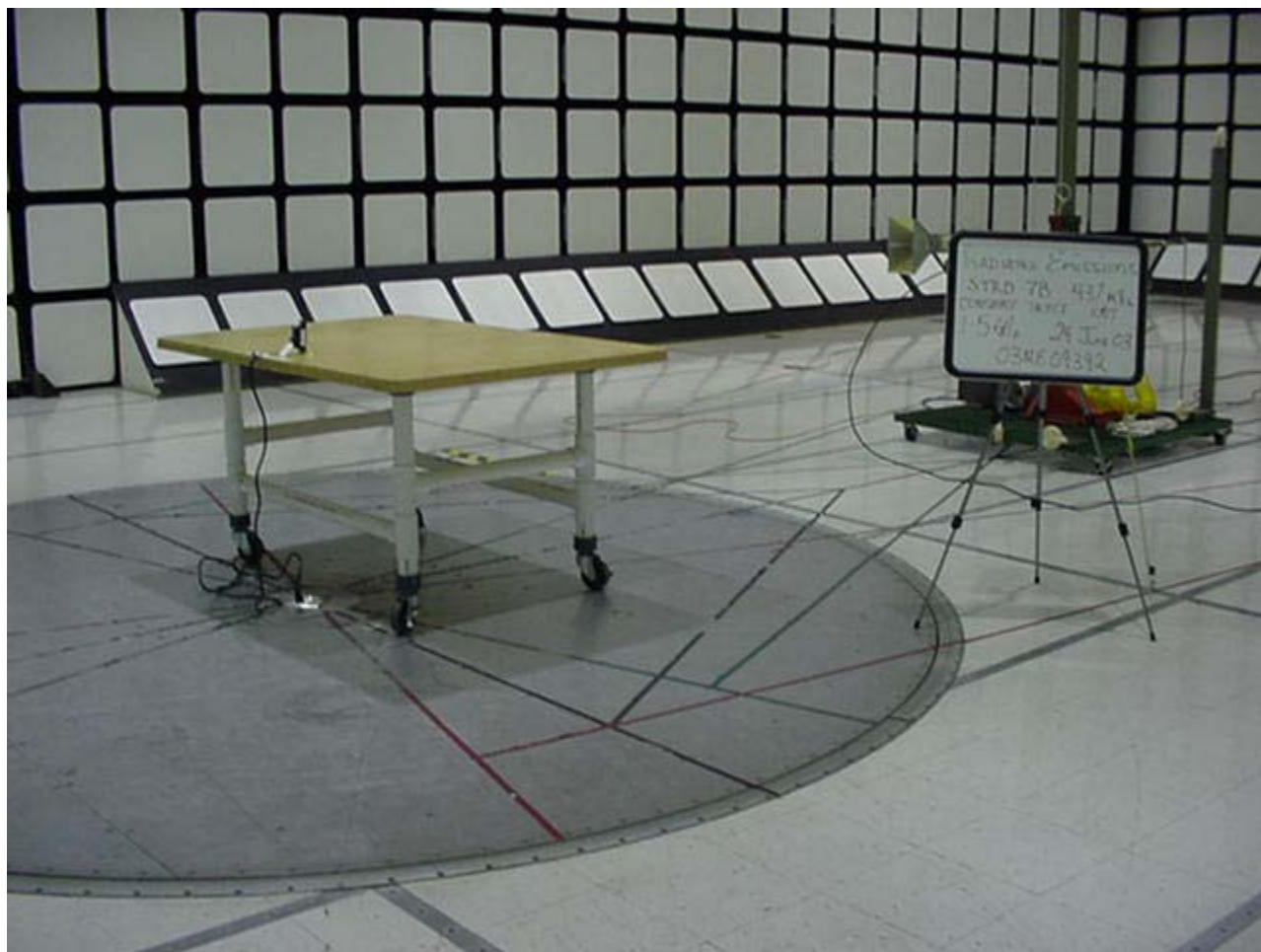
Radiated Emission Test Set-Up 1-5GHz Rear View
