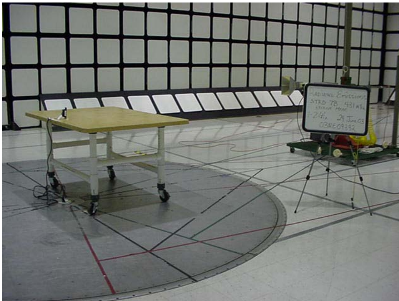
Radiated Emission Test Set-Up 1-2GHz Rear View
