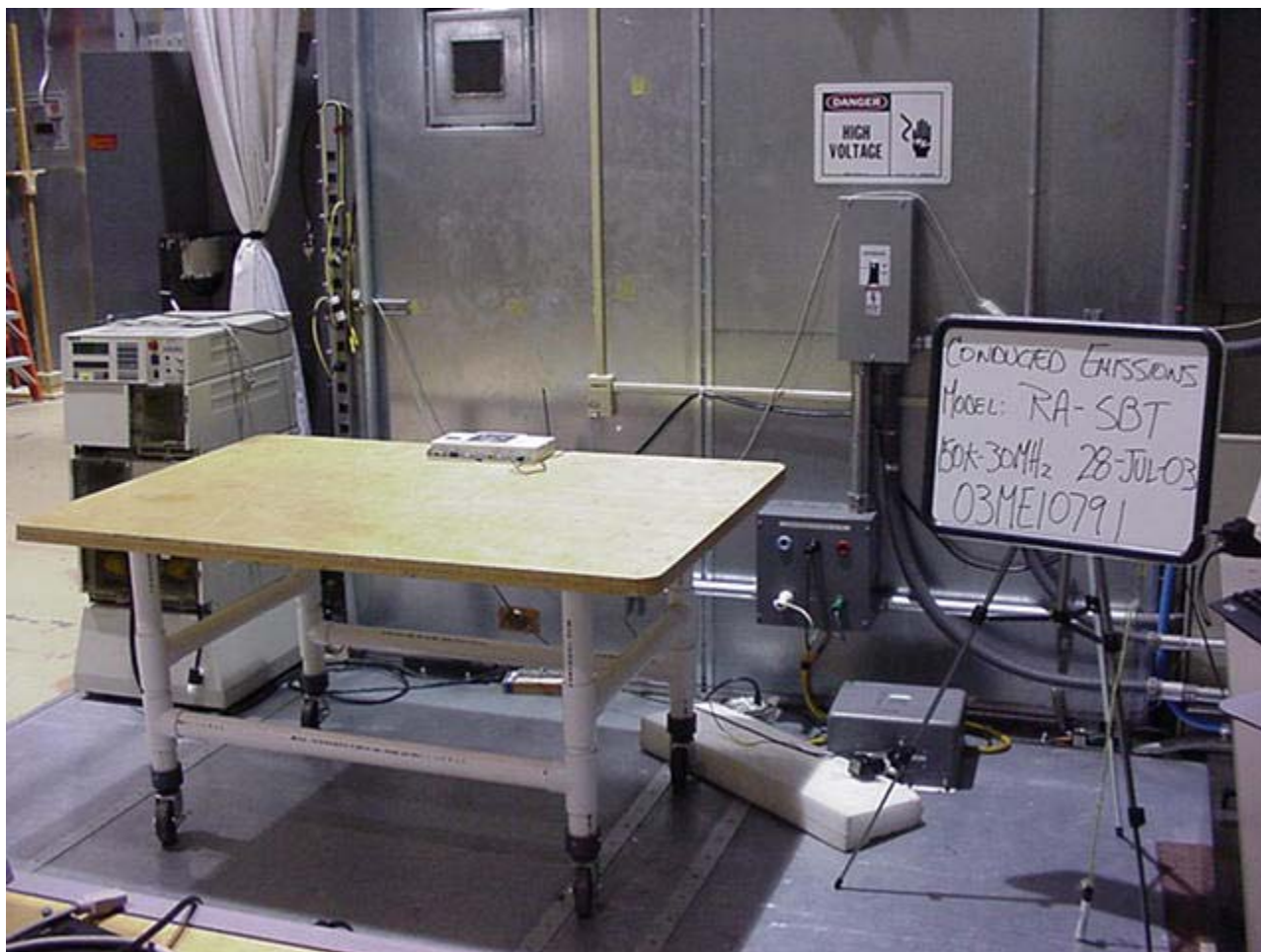
Conducted Emission Test Set-up
