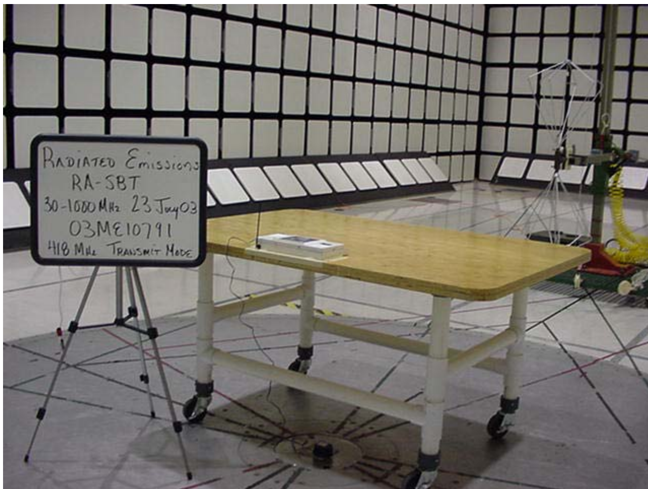
Radiated Emissions Test Set-Up
