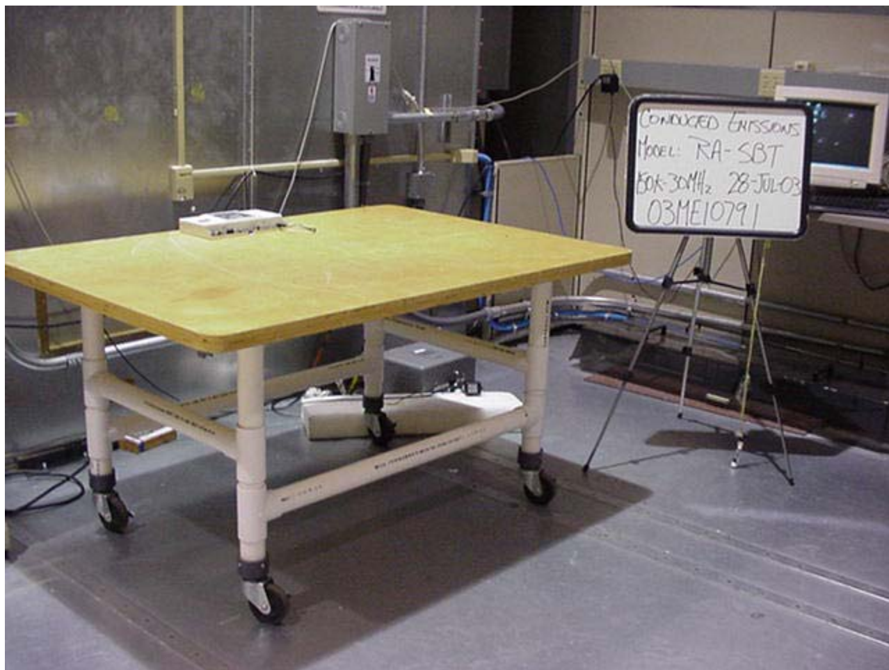
Conducted Emission Test Set-up
