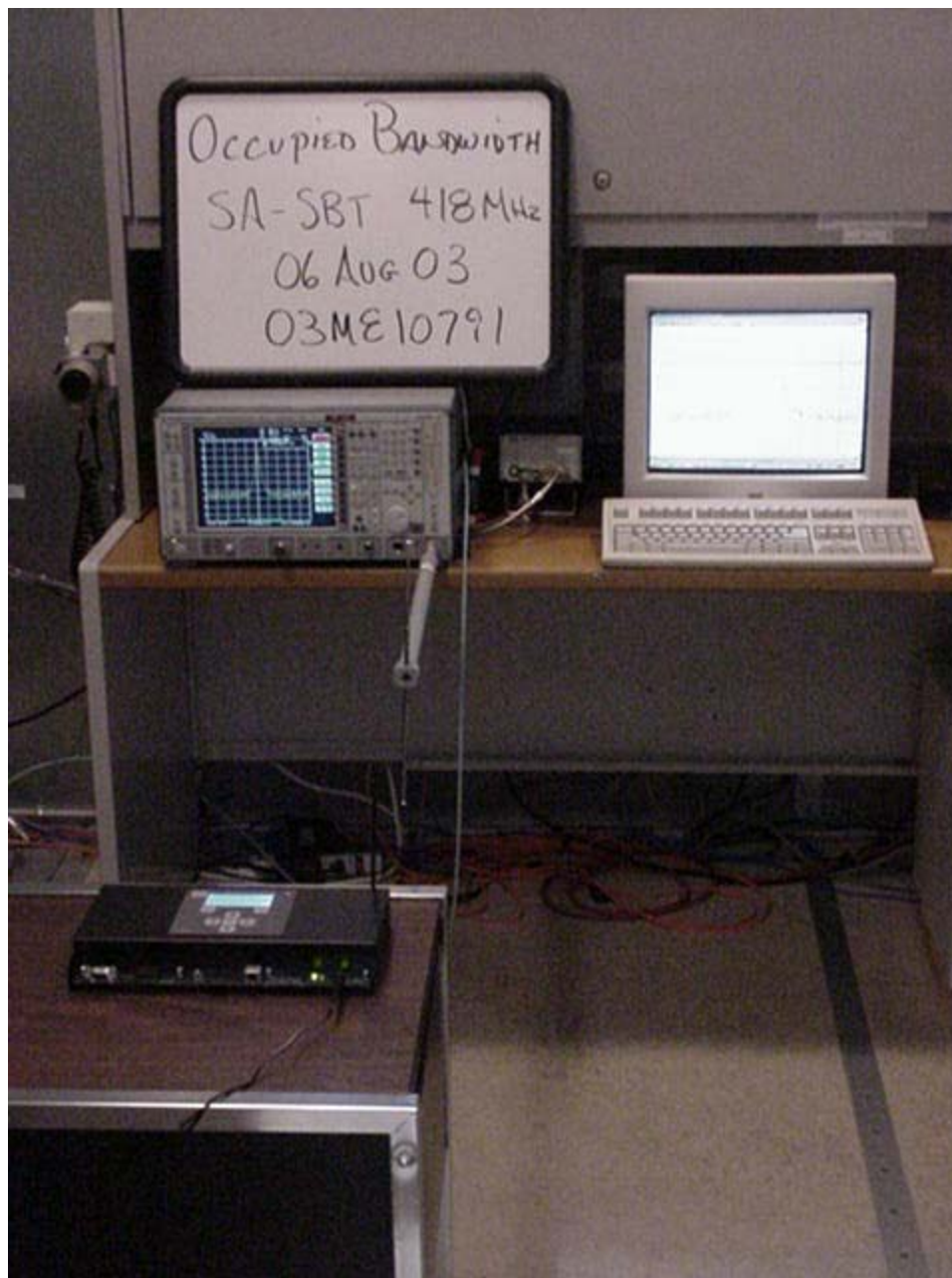
Occupied Bandwidth Test Set-up
