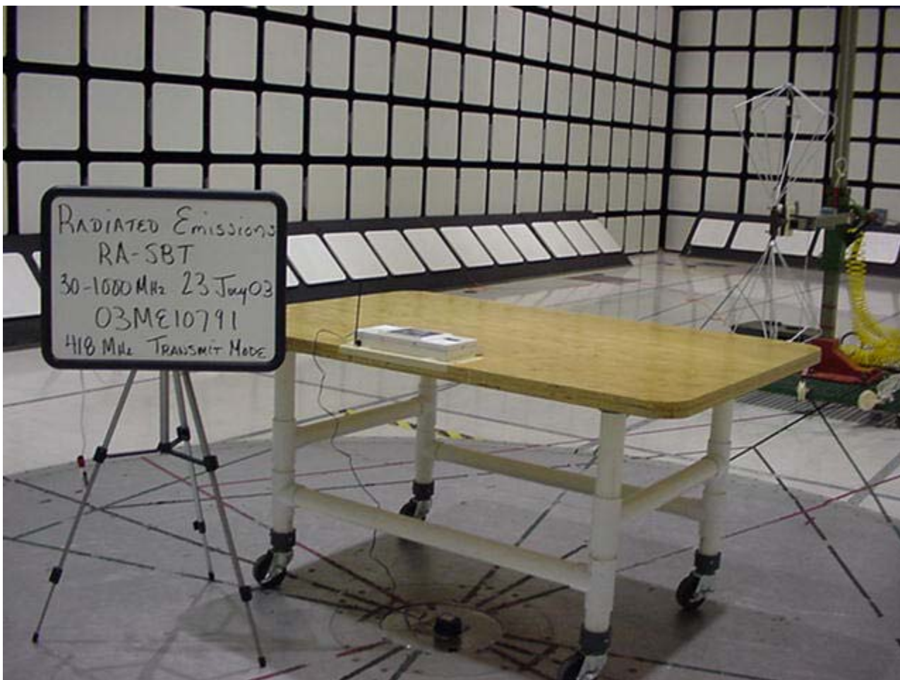
Radiated Emissions Test Set-Up
