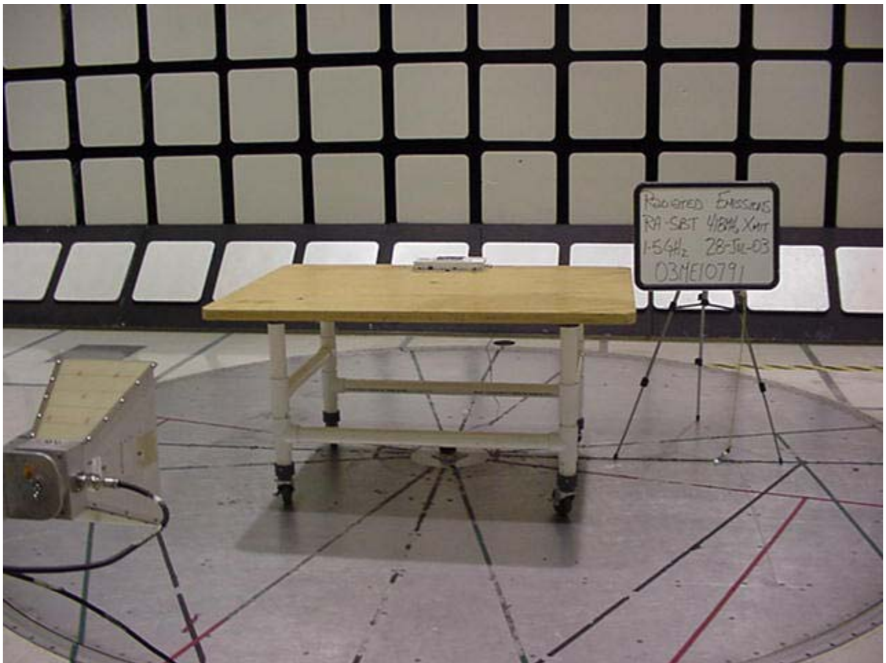
Radiated Emissions Test Set-Up
