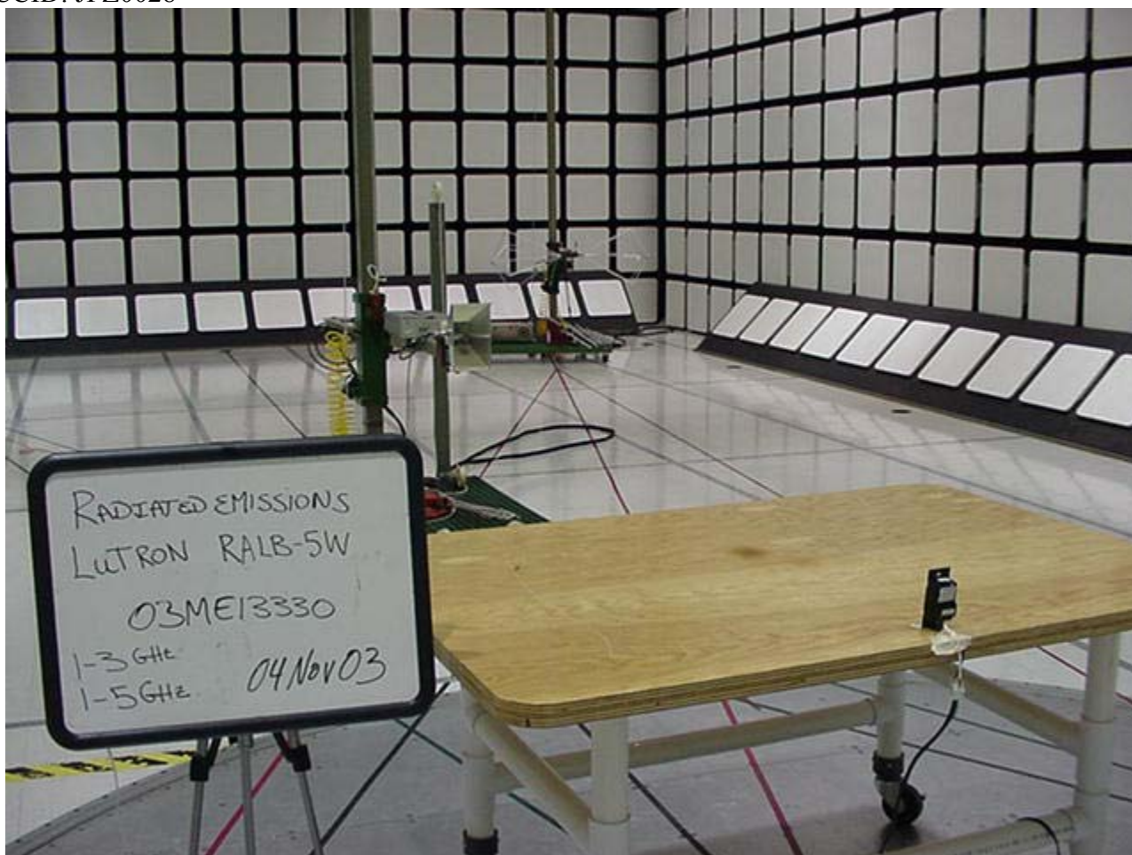
Radiated Emission Test Set-Up 1-5GHz Rear View
