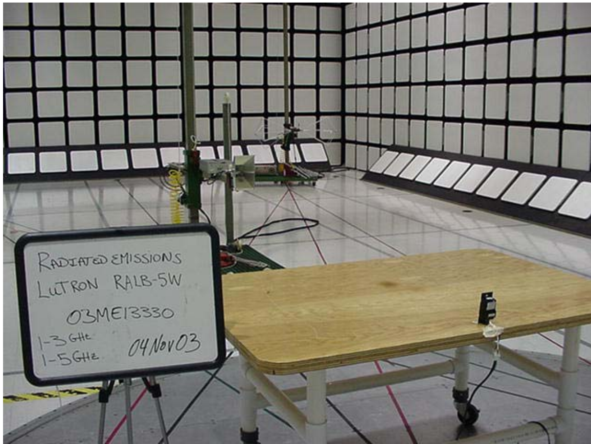
Radiated Emission Test Set-Up 1-5GHz Rear View
