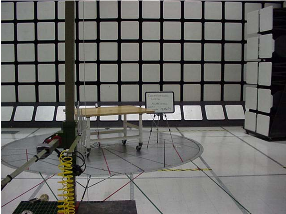
Radiated Emission Test Set-Up 200 to 1000 MHz Front View
