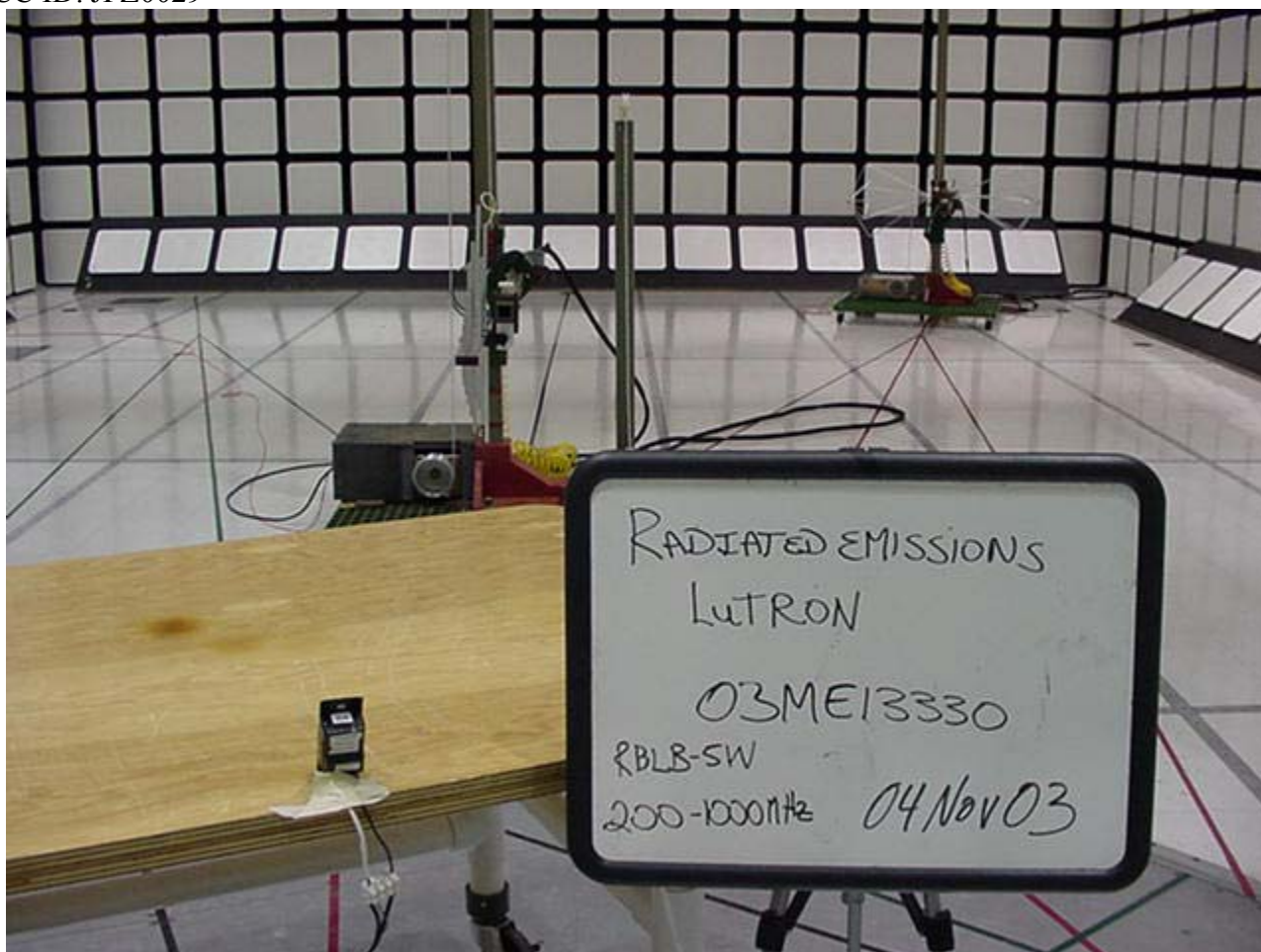
Radiated Emission Test Set-Up 200 to 1000 MHz Rear View
