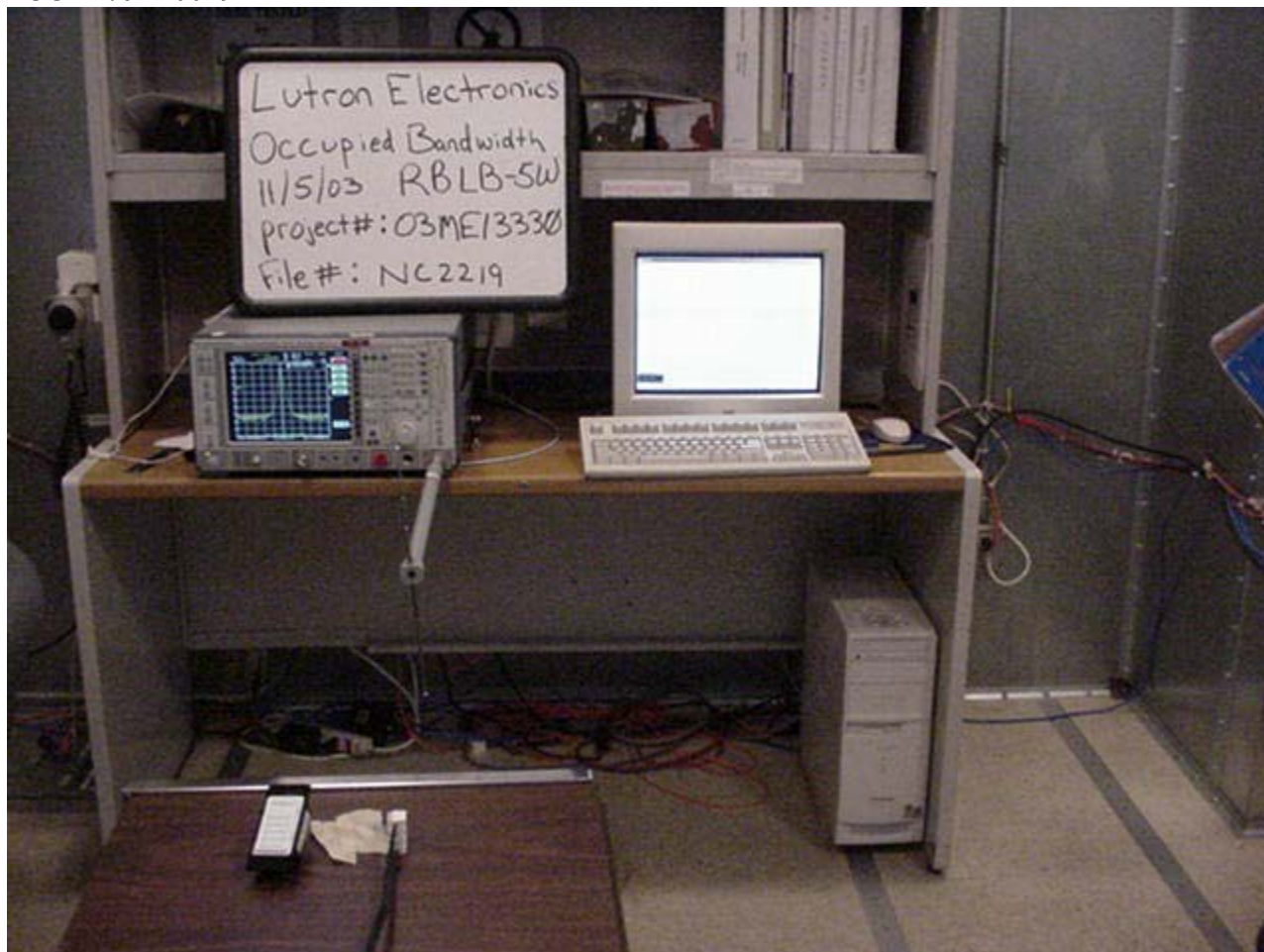
Occupied Bandwidth Test Set-up
