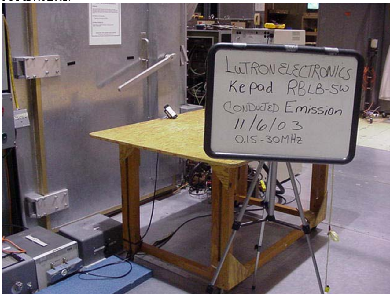
Conducted Emission Test Set-Up
