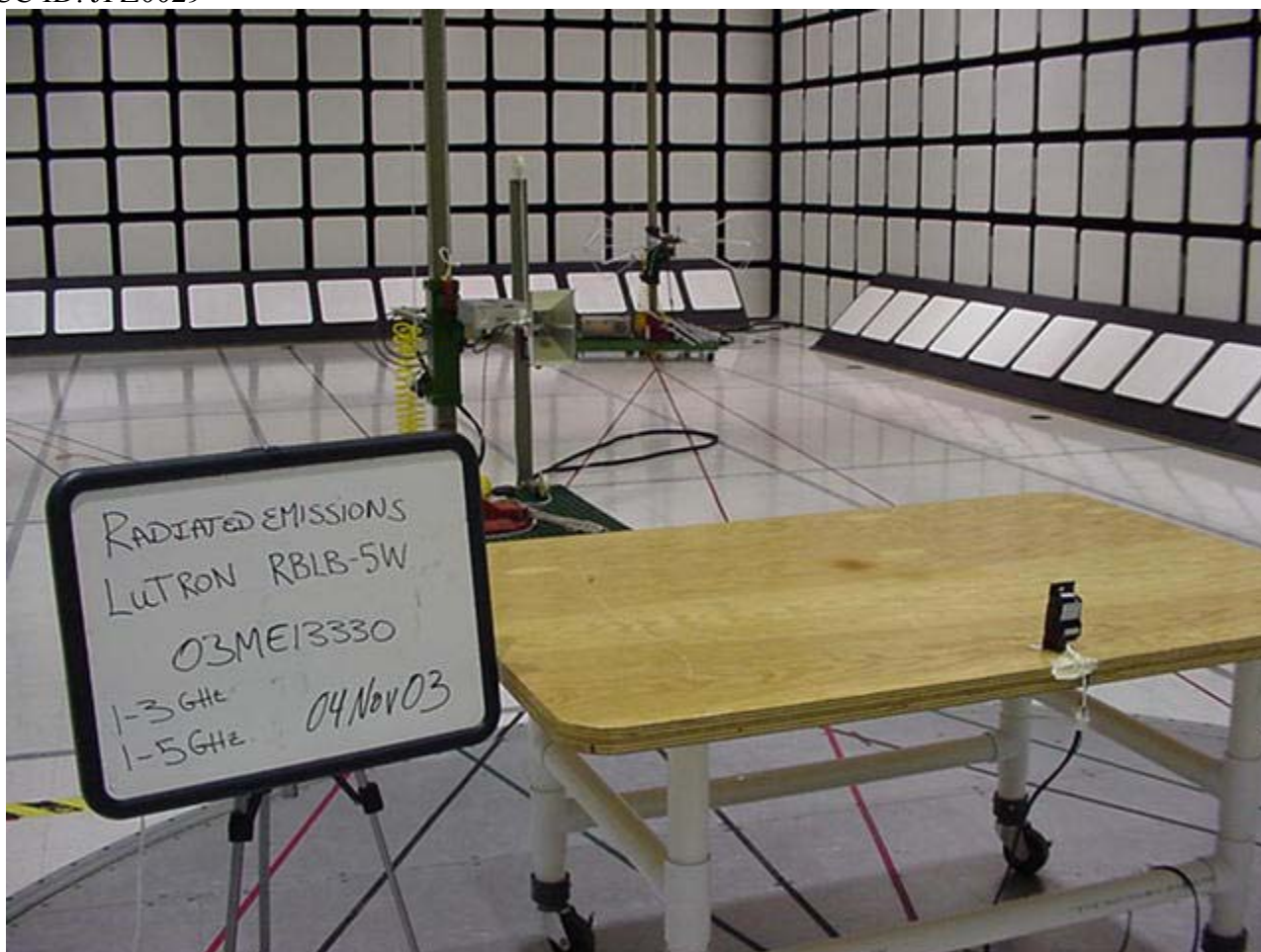
Radiated Emission Test Set-Up 1-5GHz Rear View
