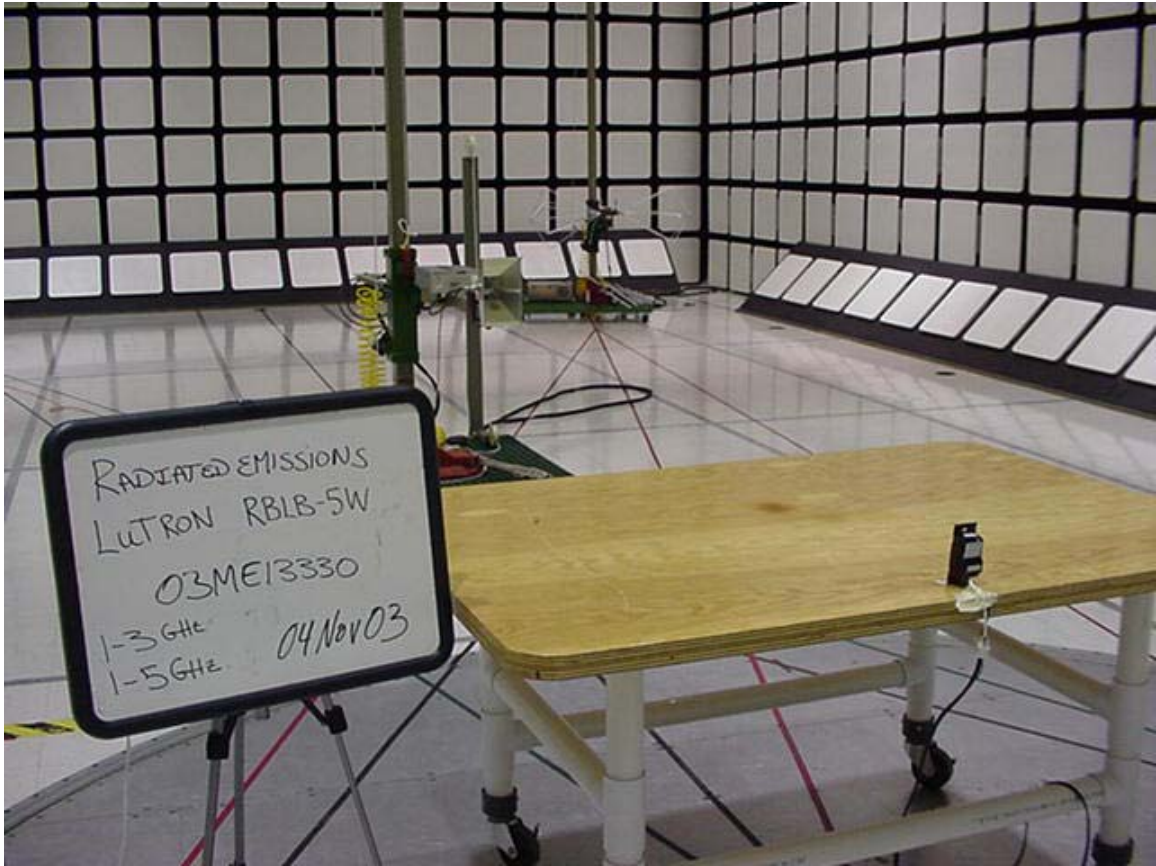
Radiated Emission Test Set-Up 1-5GHz Rear View
