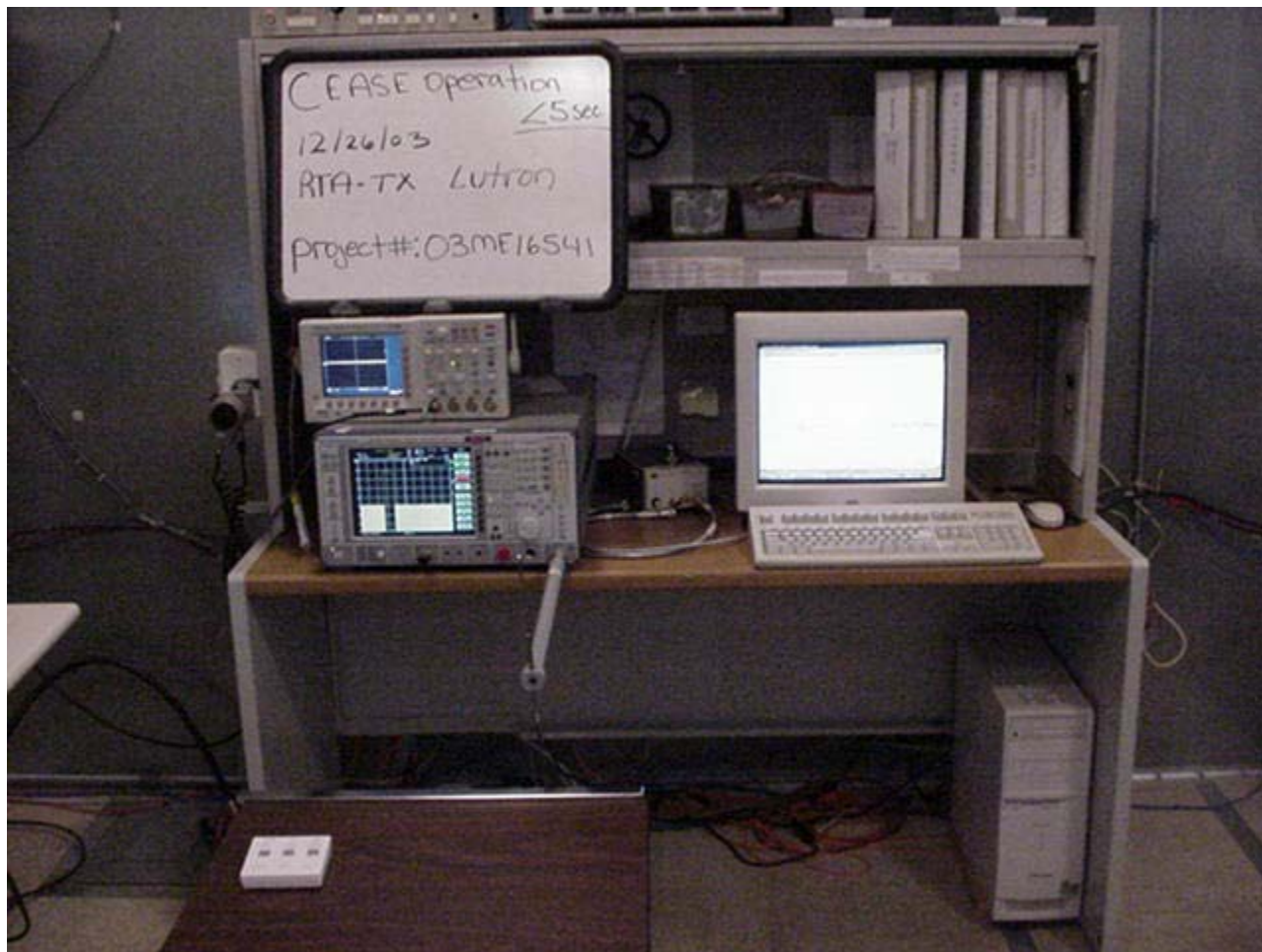
Cease Operation in < 5 Seconds Test Set- Up
