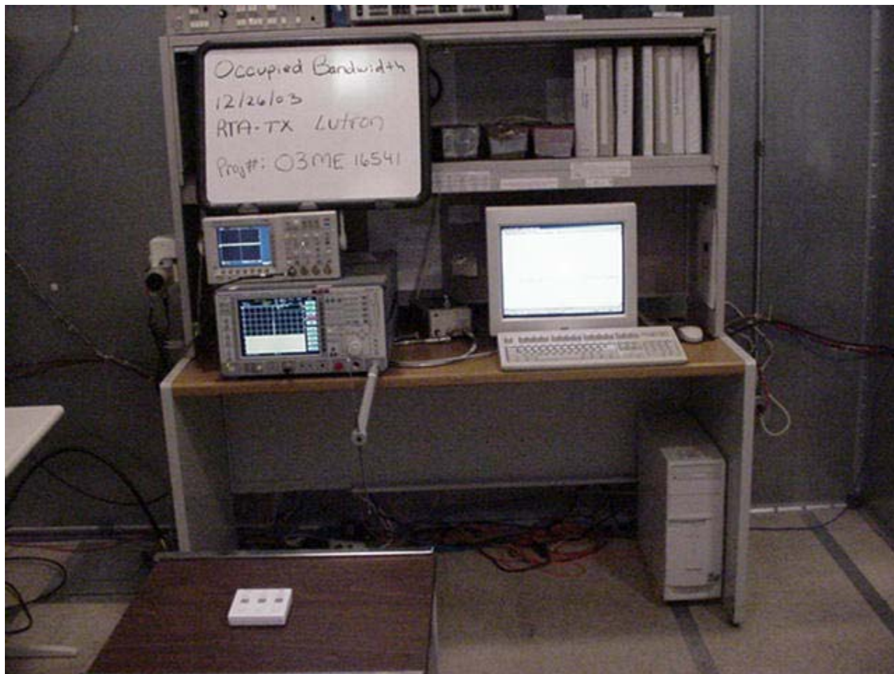
Occupied Bandwidth Test Set-Up
