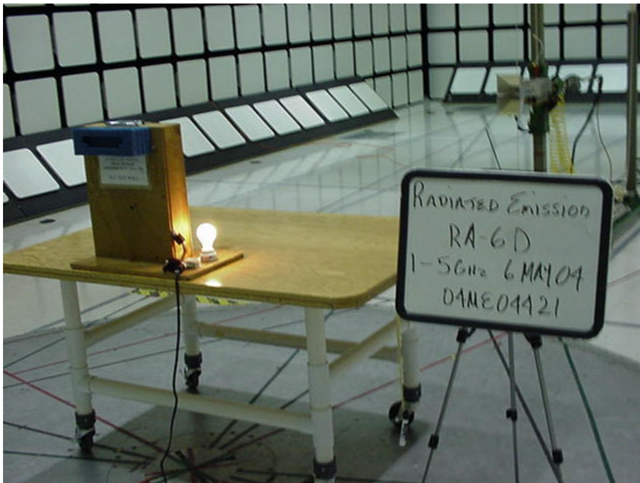
Radiated Emission Test Set-up Rear View 1-5GHz
