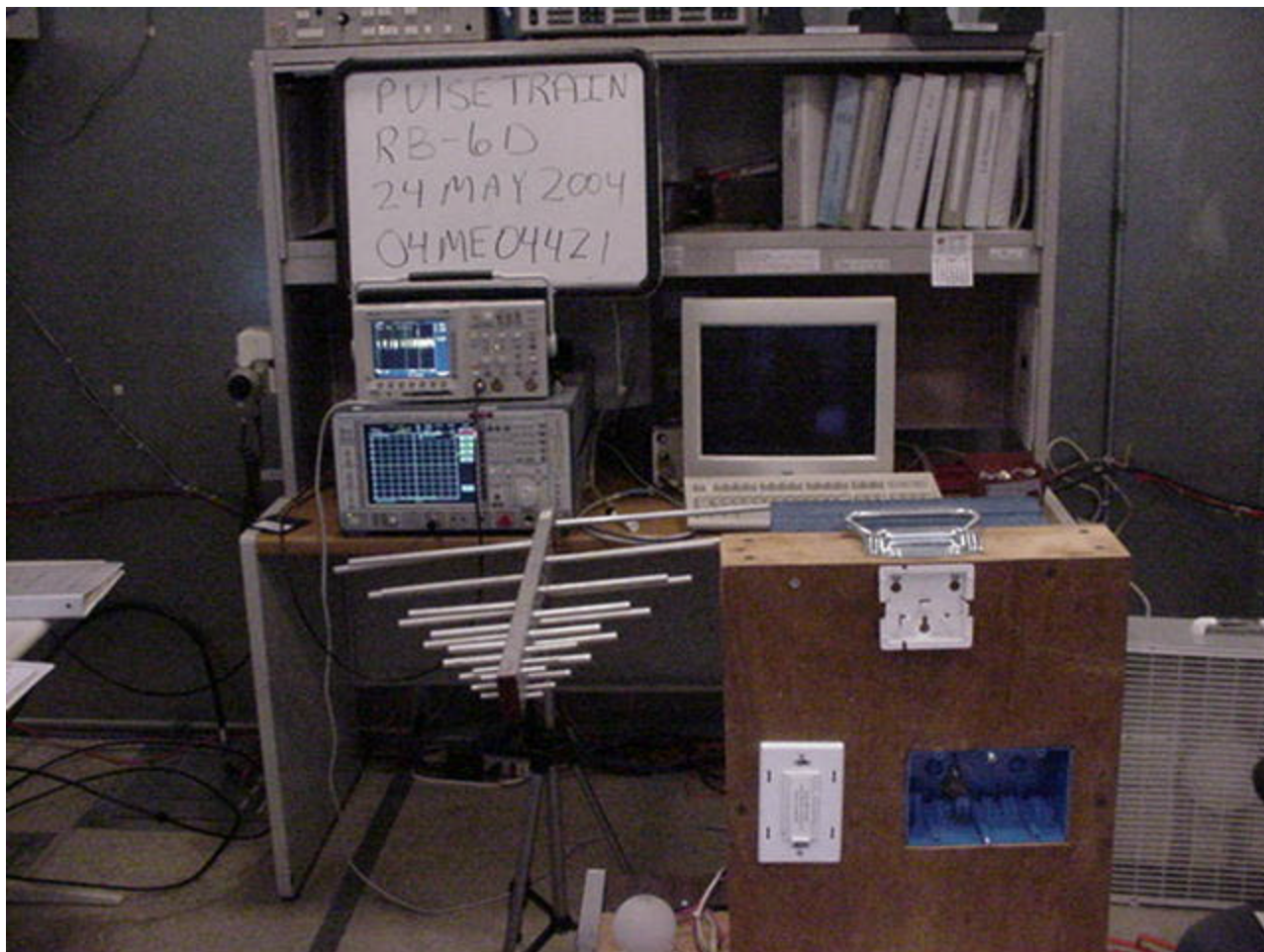
Pulse Train Test Set-Up
