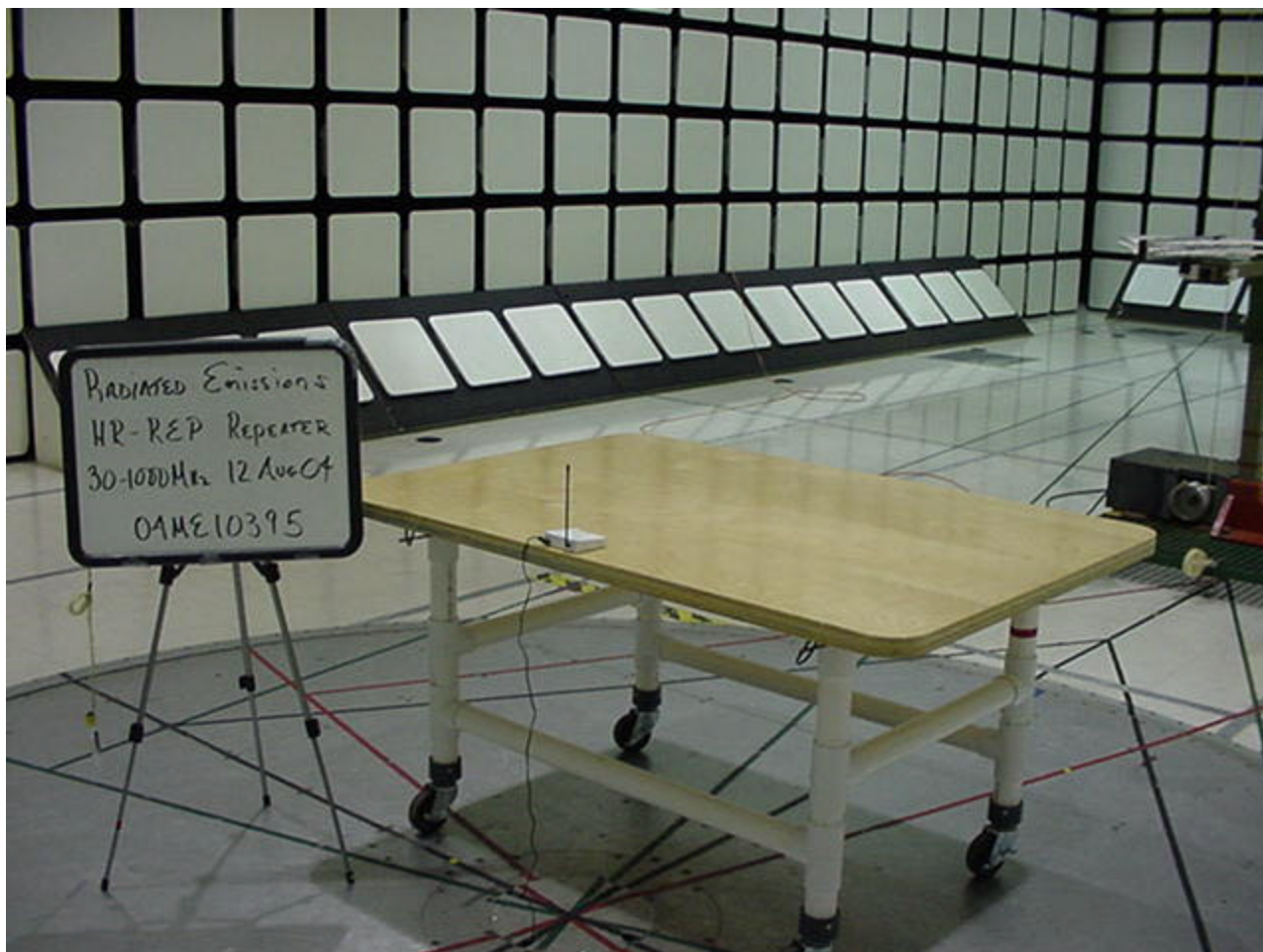
Radiated Emissions Test Set Up Rear View 30-1000MHz
