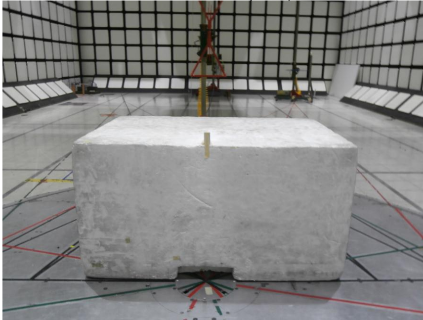
RADIATED EMISSIONS ABOVE 30 MHz (BACK)
