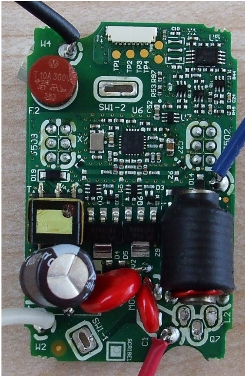
GT-RF2 Back of Power Board
