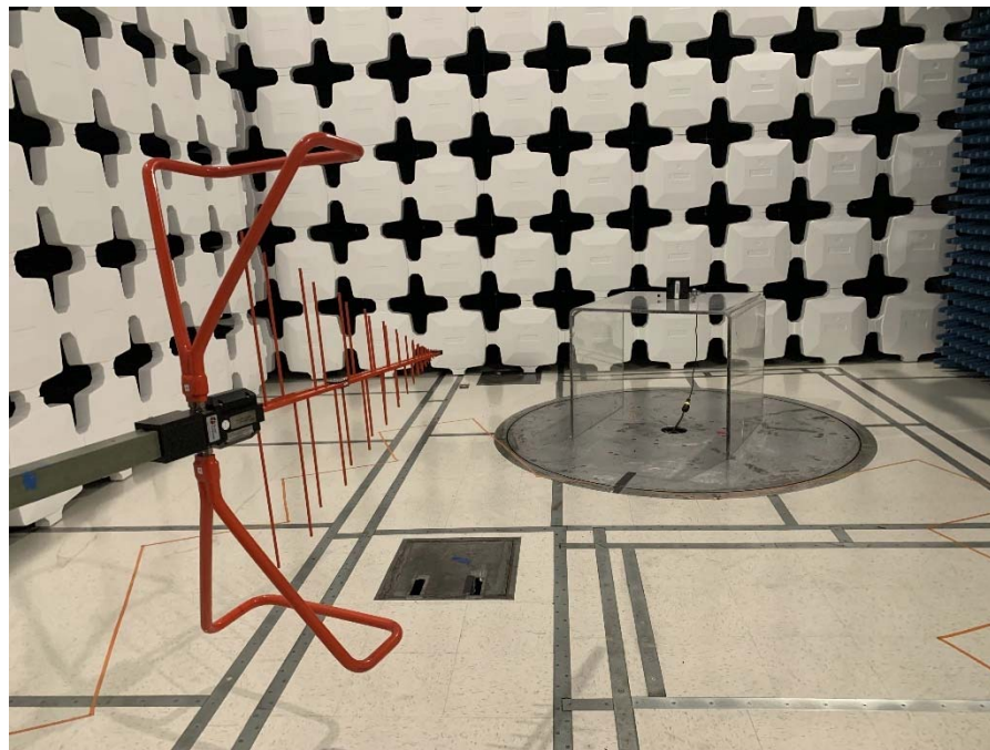
Figure 52: Cabinet Radiated emission setup 30MHz-1GHz
