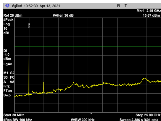
Figure 77: Conducted Spurious Emissions, BLE 1Mbit high channel
