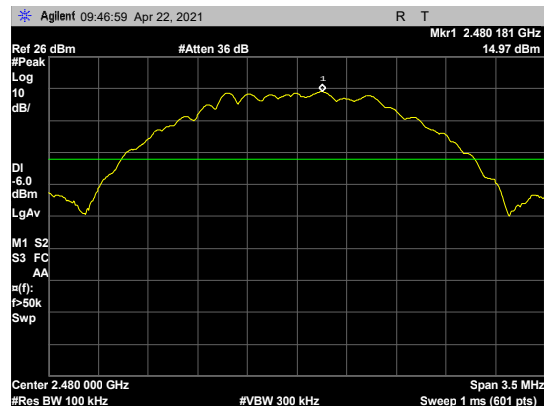
Figure 82: Conducted Spurious Emissions, BLE 2Mbit high channel reference level
