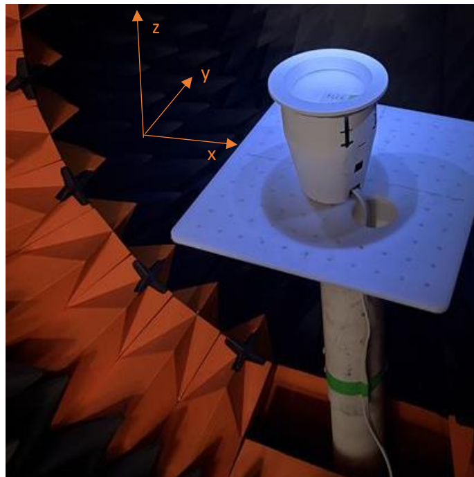
Figure 4: Antenna Gain Measurement Setup: zzz-RD4xx-yy in a 4" fixture can
