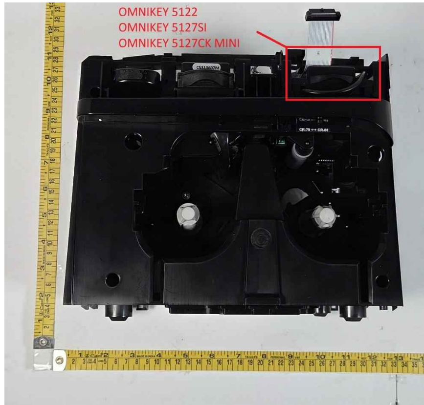
OMNIKEY (5122, 5127SI, 5127CK MINI) Antenna Location_Top of Printer
