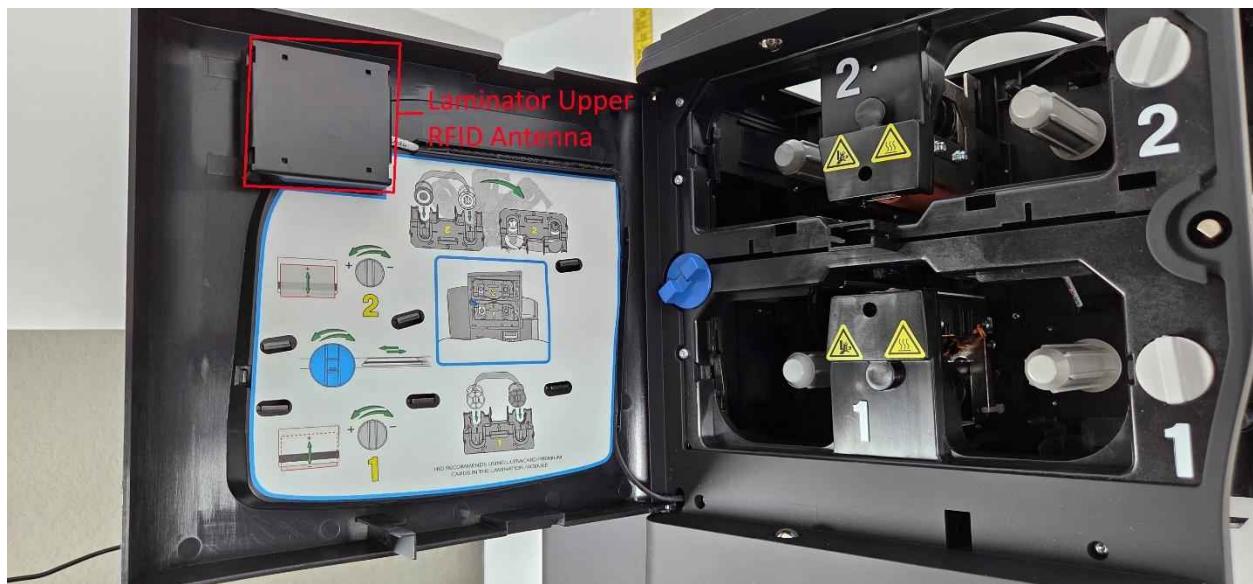
Laminator Upper RFID Antenna location – Door of Laminator
