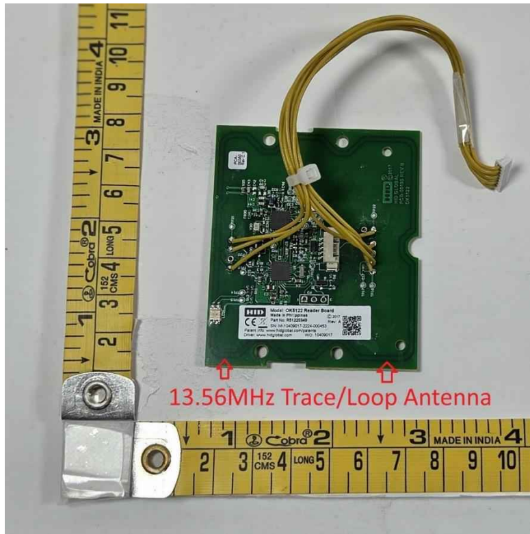
OMNIKEY 5122_HF Antenna Location_Top Side
