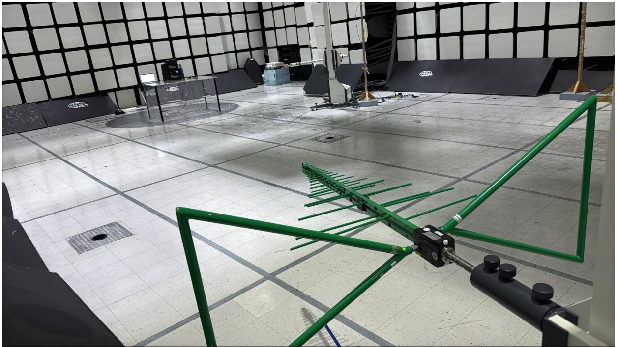
Radiated Emissions 30MHz – 1GHz Antenna View
