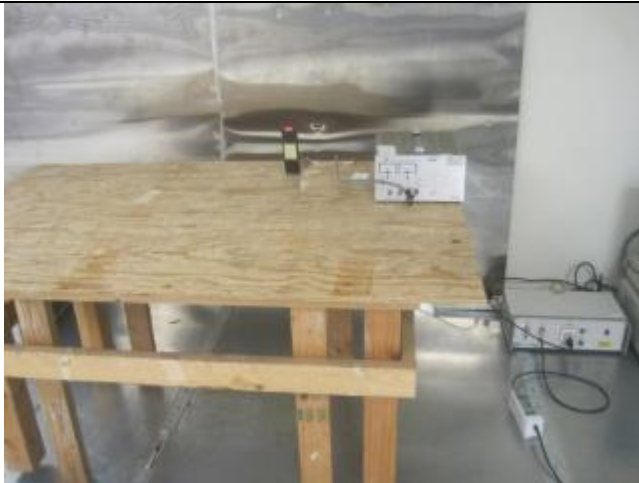
Conducted Emissions– Front View (Terminal Connector)
