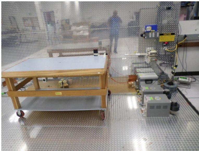
Figure 6: Conducted Emissions Limits, Terminal, Test Setup, Front View
