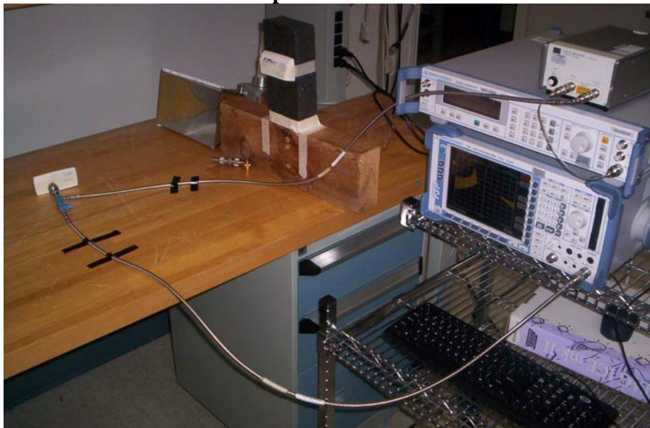
Conducted Emissions Setup:
