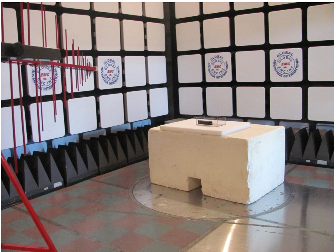
Illustration 1: Radiated emission setup – photo 1
