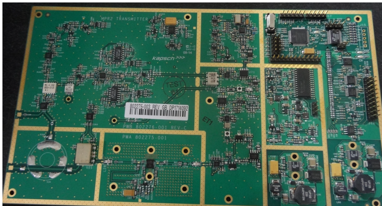
Transmitter PCA Front Photo
