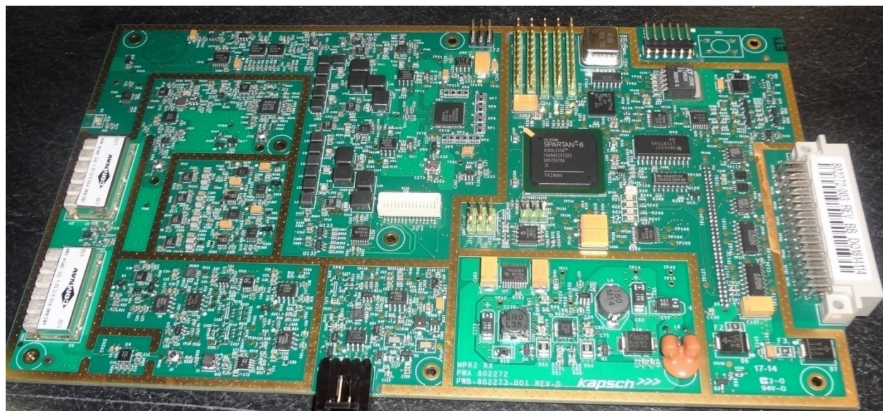
Receiver PCA Front Photo
