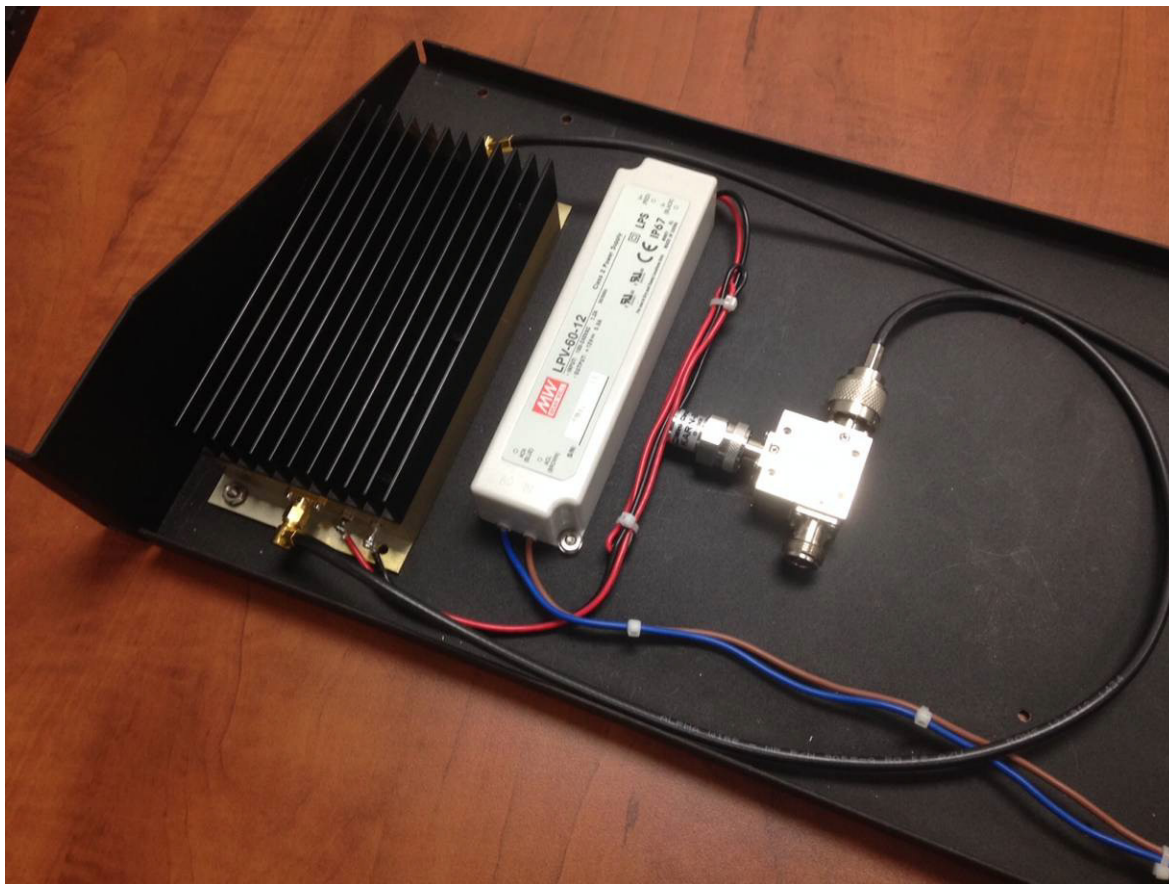
Illustration 5: 802295AA part 2 of 2, Amplifier Assembly
