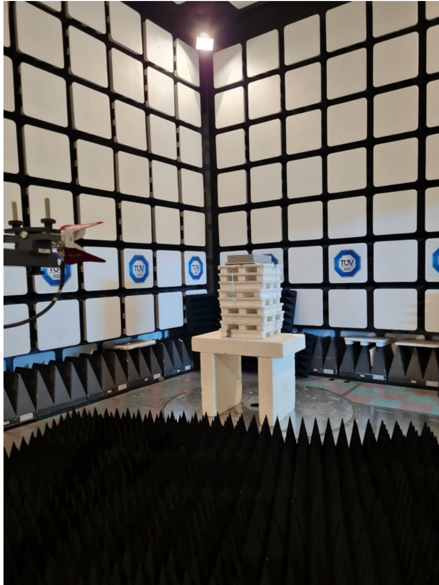
Figure 2 – Radiated Emissions Setup – Photo 2
